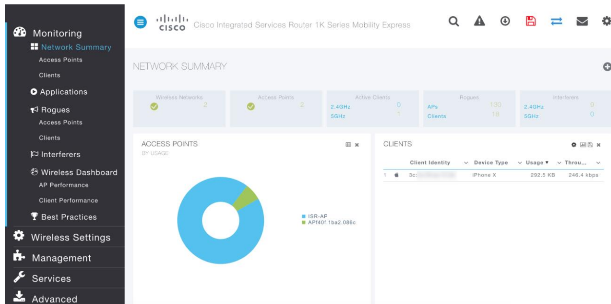
Figure 6: Cisco Mobility Express: Integrated WiFi and AP Management Interface
